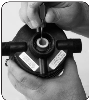
Schritt 4. Remove #82 SHAFT SEAL SPACER.
