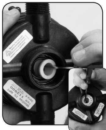
Paso 7. Replace #82 SHAFT SEAL SPACER and #16 Gasket.
