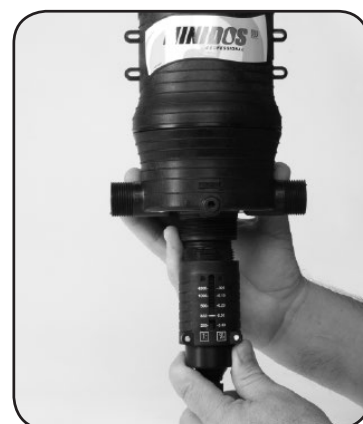
Schritt 9. Screw #7 OUTER CYLINDER onto body.
