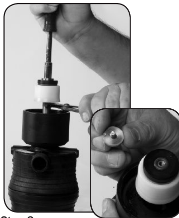
Step 2. Unscrew to unlock and remove #93 CAPSCREW.
