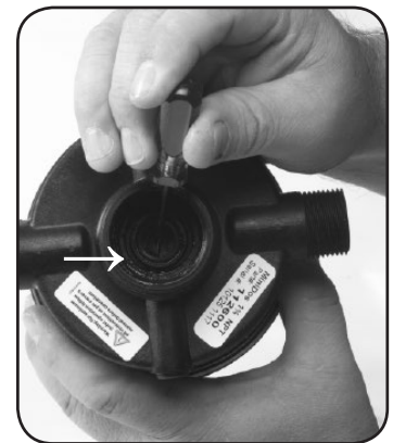
Step 6. Replace #17 O-ring.
