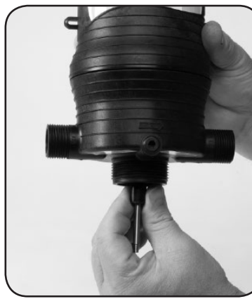
Paso 8. Replace #51 SHAFT ASSEMBLY.
