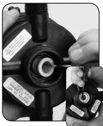
Schritt 7. Replace #82 SHAFT SEAL SPACER and #16 Gasket.
