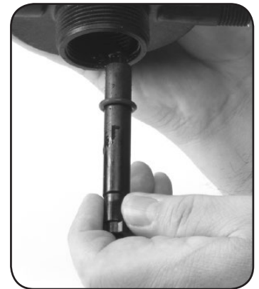
Step 6. Re-install #52 UPPER SHAFT and #17 O-ring.
