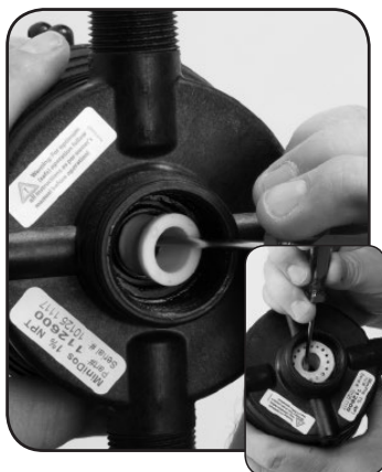
Step 7. Replace #82 SHAFT SEAL SPACER and #16 Gasket.
