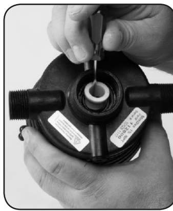
Step 5. Replace #83 SHAFT SEAL SPACER.
