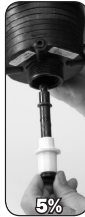
Step 2. Rotate #51 or #52 SHAFT 90° and remove.
