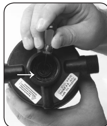
Schritt 6. Replace #17 O-ring.
