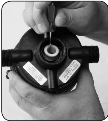
Paso 4. Remove #82 SHAFT SEAL SPACER.
