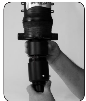
Step 9. Screw #61 OUTER CYLINDER onto body.
