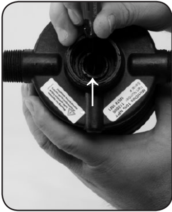
Step 4. Remove #17 O-ring and replace.
