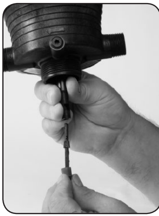
Step 2. 1/4 turn to unlock and remove #51 LOWER SHAFT and replace.
