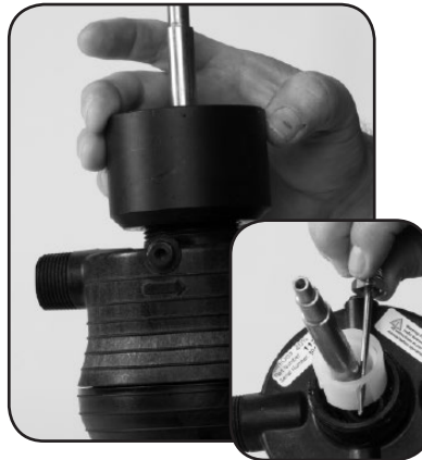
Step 5. Unscrew and remove #72 ADAPTER as well as #68 O-ring, #15 SEAL RETAINER. Clean and replace if damaged or worn.
