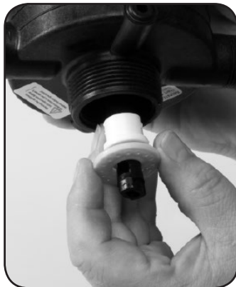
Step 7. Re-install #16 GASKET and #82 SEAL SPACER
