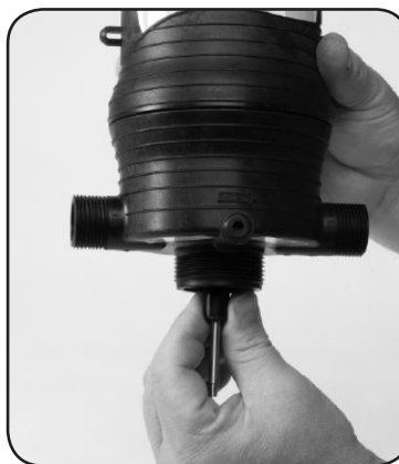
Step 8. Replace #51 SHAFT ASSEMBLY.
