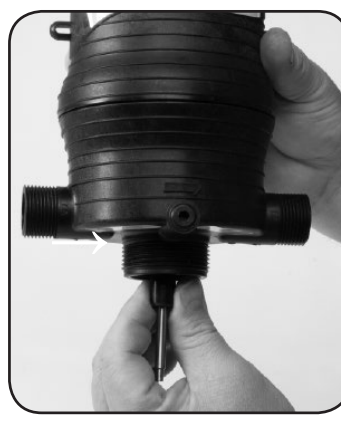
Step 6. After replacing #82 SEAL SPACER and #18 GASKET, replace #52 UPPER SHAFT. Turn 1/4 turn to lock in place.
