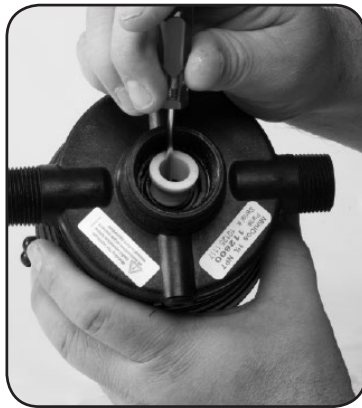
Step 4. Remove #82 SHAFT SEAL SPACER.
