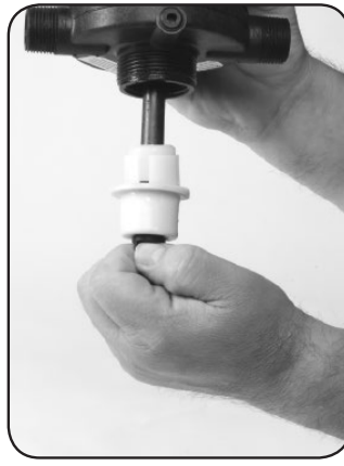
Step 2. 1/4 turn and remove #52 SHAFT, #16 GASKET and #15 RETAINER.
