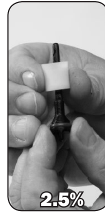
Step 3. Replace #44 DOSAGE PISTON thin lips up. Clean & inspect #14 O-ring replace if necessary.
